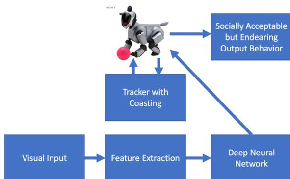
Figure 2: Object Permanence Architecture
